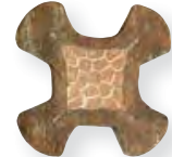
Indenter Crimp Cross-Section Across Axis
