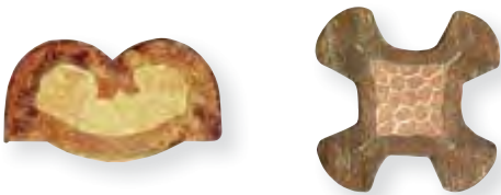
Cross section of stamped & formed and solid gas tight contact crimps
